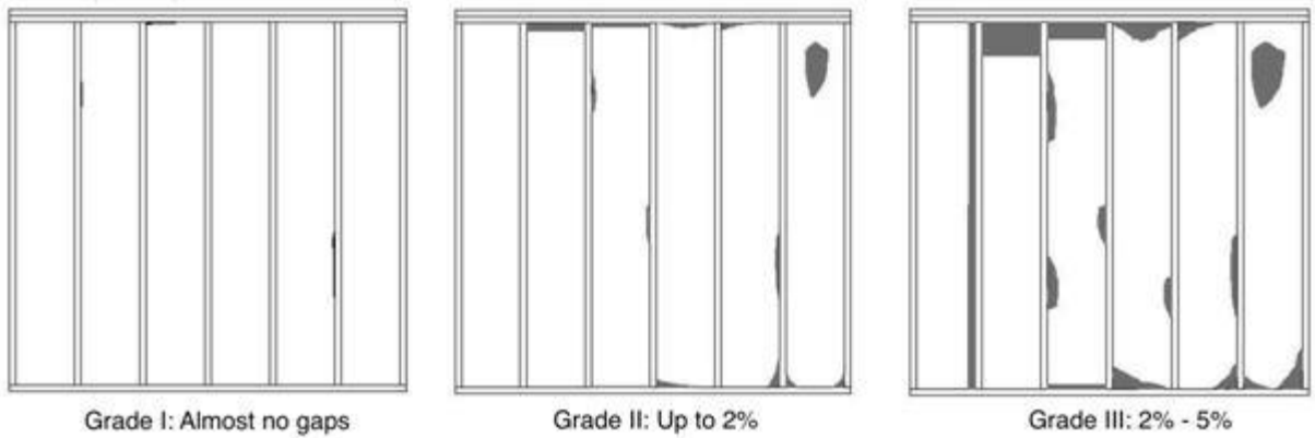
Figure 28: RESNET Protocol for Fiberglass Batt Insulation Grading
