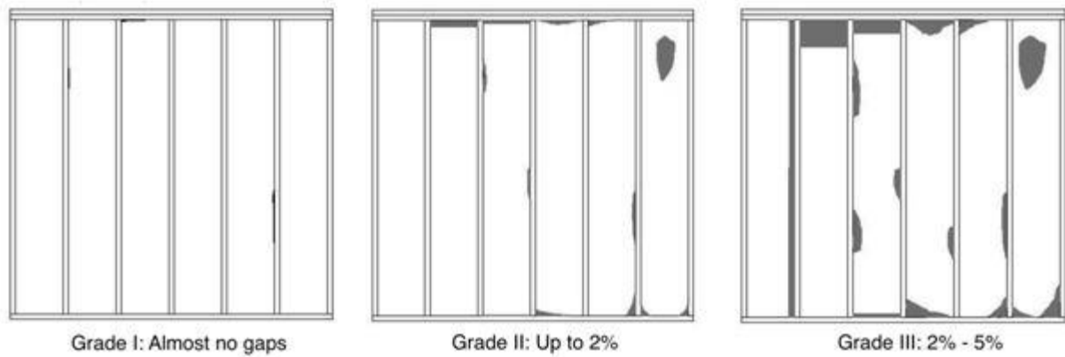
Figure 59: RESNET Protocol for Fiberglass Batt Insulation Grading
