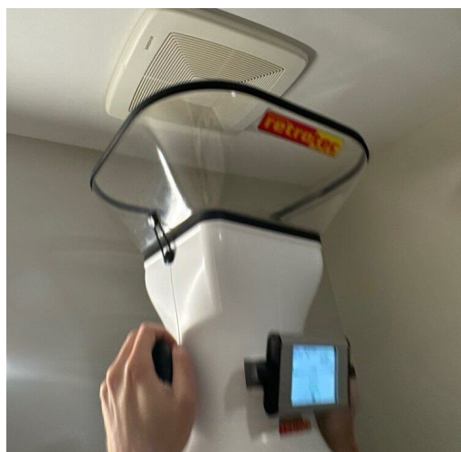
Figure 2: Measuring exhaust fan airflow with a balometer
