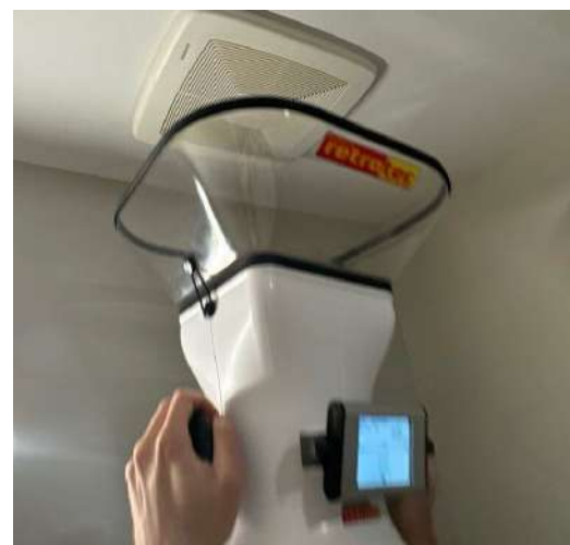
Figure 2: Measuring exhaust fan airflow with a balometer
